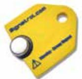
The loggers are self contained, sealed units capable of taking 8000 readings (~43 Days of logging at 15minute intervals). If you require longer periods of operation please look at our Tinytag range of data loggers. The loggers come with calibration certificate and are calibrated to ±0.5°C and ±2%RH, loggers can be re-calibrated at additional cost.
