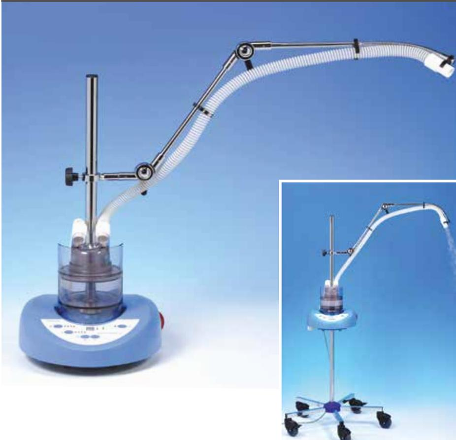
The Reco 100 heated Aerosol Generator is ideal for various conservation and restoration techniques where atomisation, humidification or non-contact application are required. The heated hose fitting contains a spiral heating element, allowing aerosol contents to be heated up to 43°C.
